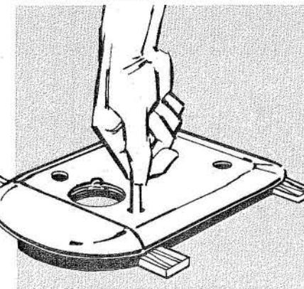
Place plate on blocks and press out roller shell from ring assembly, as shown.
